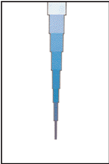
Fig. 7.5.1 A conical point can be regarded as a series of cylindrical electrodes of increasing diameters. At the tip, where the diameter is smallest, the current density, and therefore the lesional effect, is greatest.
