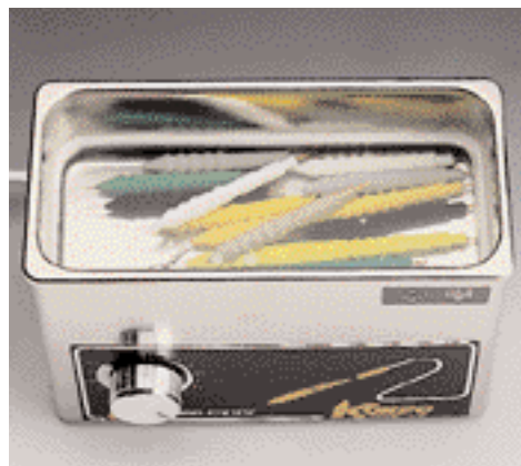
Fig. 13.2.3 Ultrasonic bath. Clean cables and electromaniples in a detergent for 15 minutes.
